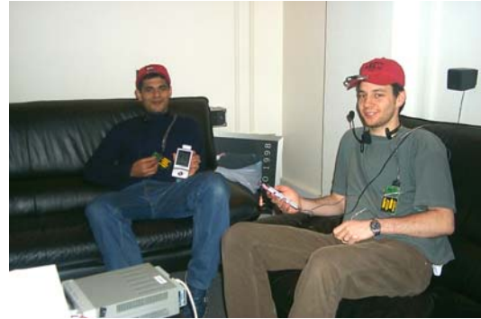
Fig 2: The present system featuring a Zaurus PDA, Hoarder sensor board, bluetooth accelerometer (on hat), GSR leads and a microphone
