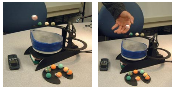
Figure 1: At Jane’s end, a ball floats when a call comes in. She grabs the ball to answer the call.
